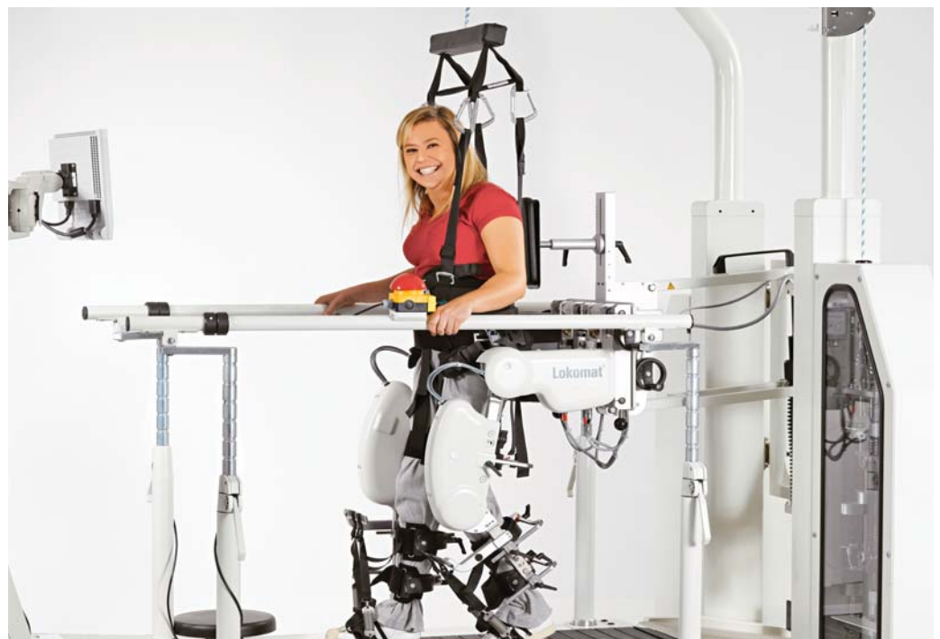
The Lokomat® – a robotic gait exoskeleton, body weight support system, treadmill, and screen mounted at eye level to provide patient with motivation. (Picture courtesy of Hocoma.)
