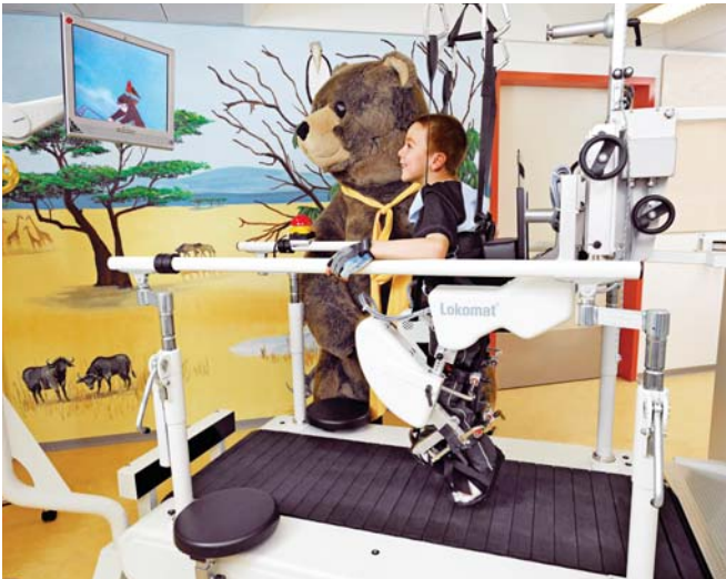
FIGURE 2 (above): Unloading of body weight during training by the Lokomat® body weight support system – the Levi. (Picture courtesy of Hocoma.)
